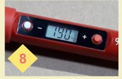
Set the temperature in the soldering iron
