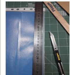
Make the last cut at the top, 5mm from the edge of the envelope
