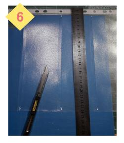
First, cut in the marked area, then the second cut next to it, approx. 7-10mm
